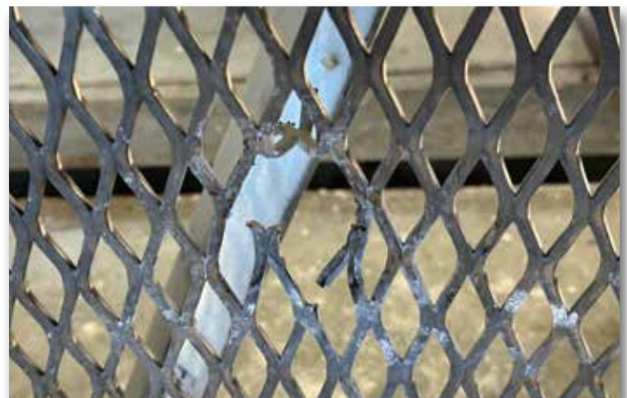
AMICO Security Mesh™ at test termination after 600 impacts achieving Grade 1
